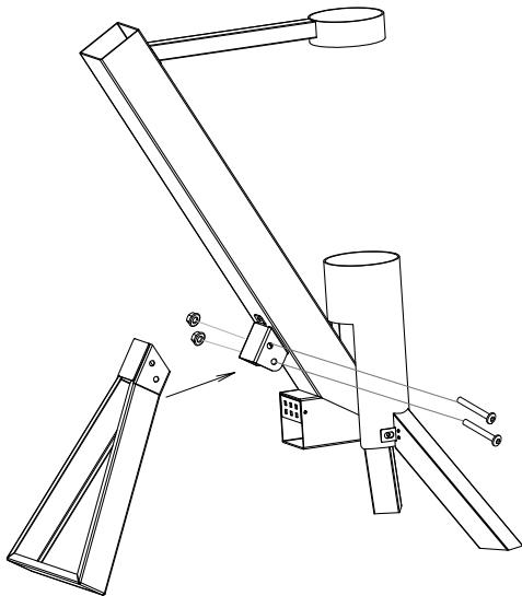
**Step 4** Insert the support leg 2 into the rocket body support and tighten with long screws and bolts (pay attention to the level adjustment).
