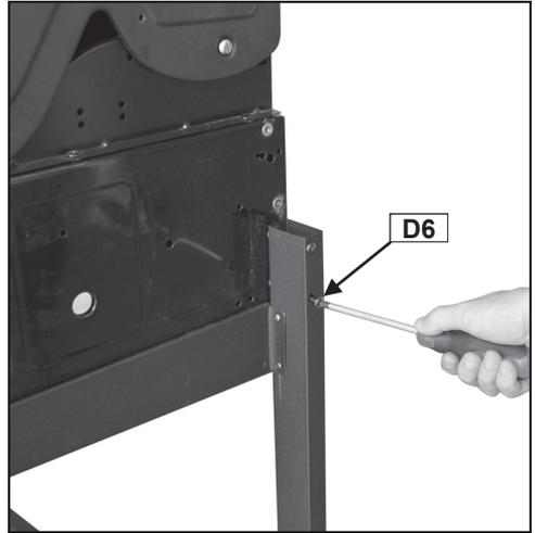
Carefully place the Barbecue Body (B1) onto the trolley assembly and fix using M6x65 Bolts (D6x8pcs) as shown.
