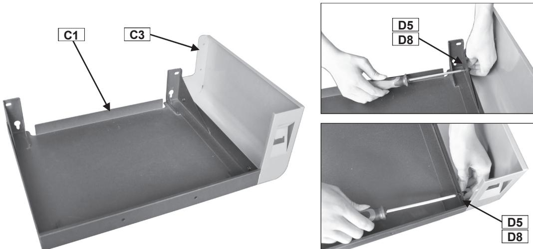
Attach the Right Side Shelf Panel (C3) onto the other Side Shelf (C1) using M6x15 Bolts (D5x2pcs) and M6 Nuts (D8x2pcs).
