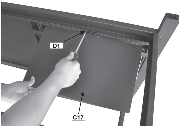
Attach the Charcoal Bin Lid (C17) onto the front support using ST4.0x10 Screws (D1x3pcs) as shown.
