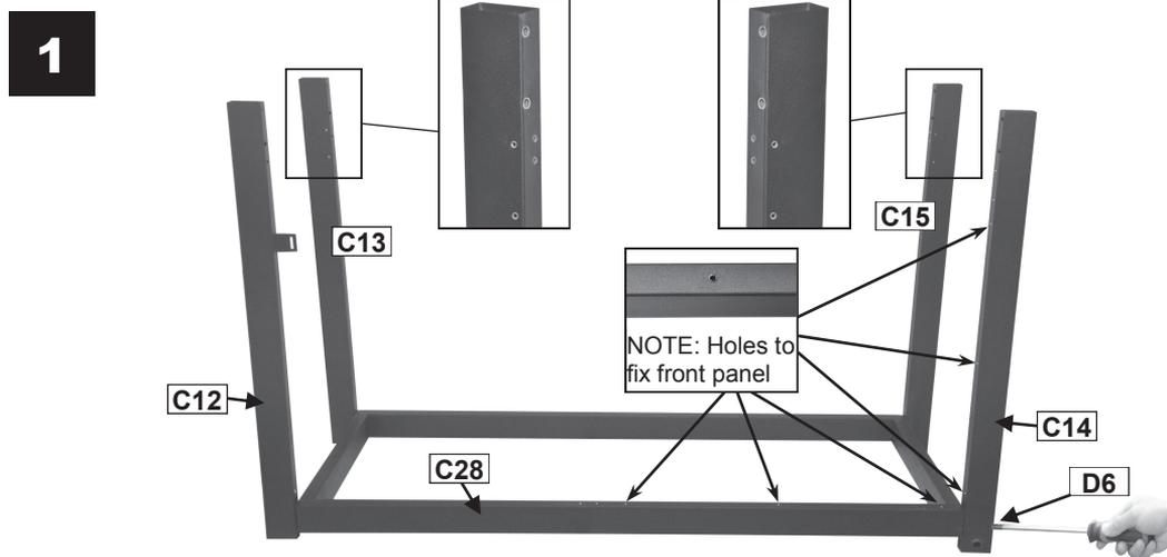
Attach the Left Legs (C12, C13) and Right Legs (C14, C15) to the Underframe (C28) using M6x65 Bolts (D6x8pcs) as shown.
