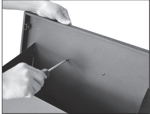
Remove retaining bolts from the Charcoal Bin Handle (C22), and then attach the handle onto charcoal bin front panel using the retaining bolts.
