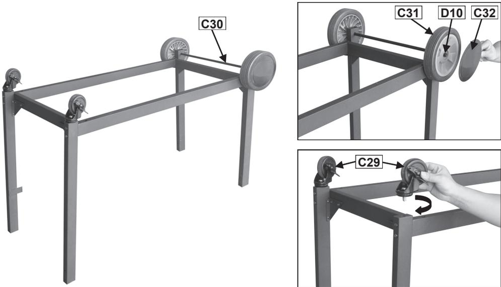
Unscrew the Locknuts (D10) from both ends of the Axle (C30).
