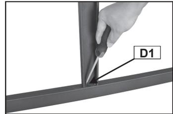
Attach the Front Trim Panel (C24) between the front support and underframe using ST4.0x10 Screws (D1x4pcs) as shown.
