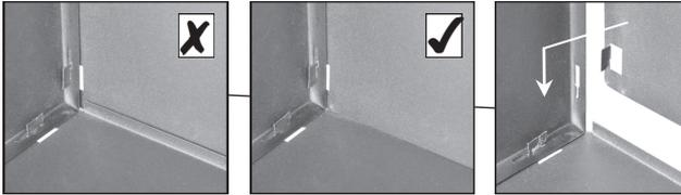
Attach the Charcoal Bin Left Side Panel (C20) and Charcoal Bin Right Side Panel (C21) onto the Charcoal Bin Back Panel (C18) by inserting the locking tabs of back panel into the slots on side panels and sliding to the end; then install the Charcoal Bin Bottom Panel (C19) into place as shown.
