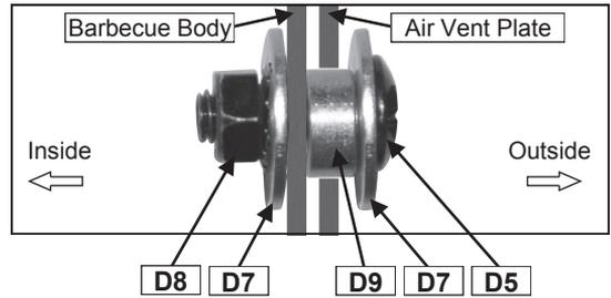
Attach the Air Vent Plate (B7) to the barbecue body using M6x15 Bolts (D5x4pcs), Spacers (D9x4pcs), Ø6 Washer (D7x8pcs) and M6 Nuts (D8x4pcs) as shown.
