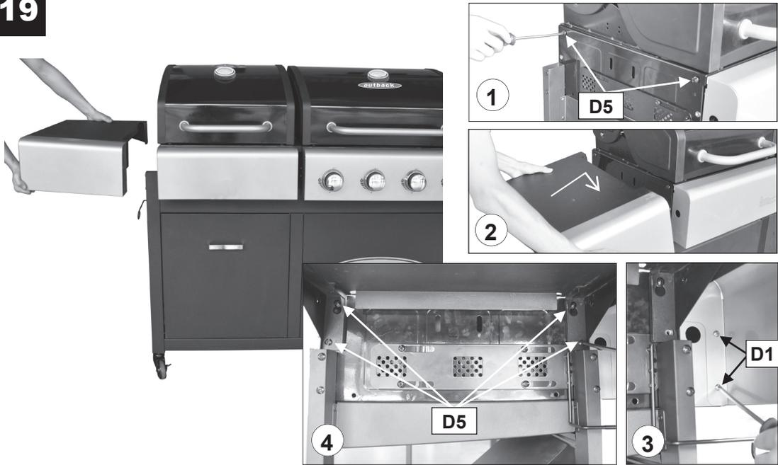
Attach the left side shelf assembly to the barbecue body using ST4.0x10 Screw (D1x2pcs) and M6x15 Bolts (D5x4pcs) as shown.
