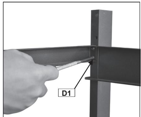
Attach the Rear Support (C4) between the rear legs using ST4.0x10 Screws (D1x4pcs) as shown.
