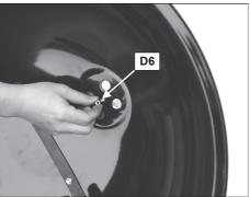
Attach the Air Vent (A4) onto the Hood (A1) using the M5x12 bolt (D5x1pc) and  $\,$  M5 Nut (D6x1pc) as shown.
