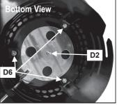
Attach the Ash Tray Bracket Assembly onto the Barbecue Body (B1) using the M5x12 bolts (D5x3pcs) and M5 Nuts (D6x3pcs) as shown.
