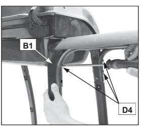
Attach the left side shelf assembly to the Left Arch Support (B1) using M6x15 Bolts (D4x3pcs) as shown. Repeat above process to install the right side shelf assembly to Right Arch Support (B2) using M6x15 Bolts (D4x3pcs).
