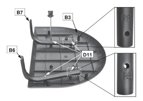
Attach the Side Shelf Right Front Bracket (B7) and Side Shelf Right Rear Bracket (B6) onto one Plastic Side Shelf (B3) using ST4.8x35 Screws (D11x4pcs) as shown.
