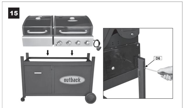
Carefully place the Barbecue Body (B1) onto the trolley assembly and fix using M6x65 Bolts (D6x8pcs) as shown.
