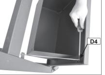
Insert one tip of Charcoal Bin Slider (C16) through the left front leg, and fix another tip of the slider onto charcoal bin front panel using a M6x15 Step Bolt (D4) as shown.
