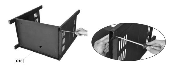
Attach the left / right cabinet panel assembly to the Bottom Panel (C18) using M6x40 Bolts (D5x8pcs) and M6 Nuts (D6x8pcs) as shown.
