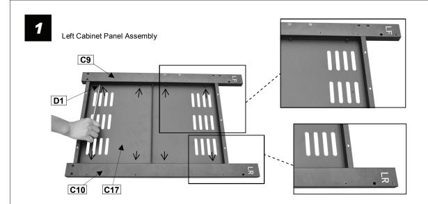
Attach the Left Legs (C9,C10) to the Side Panels (C17x2pcs) using ST4.0x10 Screws (D1x8pcs) as shown.
