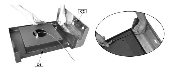
Attach Side Burner Shelf Panel (C2) onto Side Burner Shelf (C1) using M6x15 Bolts (D4x2pcs) and M6 Nuts (D6x2pcs).
