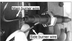
Connect the electrode wire to the Ignition Button (B13).
