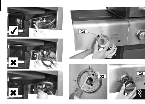
Attach the side burner valve and Knob Bezel (C4) onto side burner shelf using M4x10 Bolts (D2x2pcs) as shown. Press the Side Burner Knob (C5) onto side burner valve stem.
