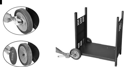
Unscrew the Locknuts (D7) from both ends of the Axle (C21).
