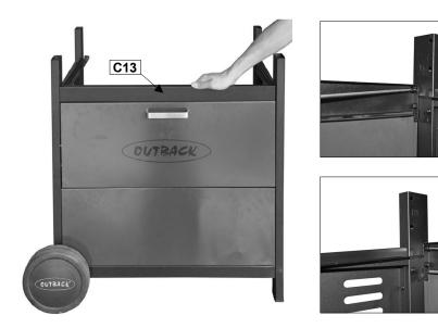
Attach the Upper Support (C13) to the front legs using M6x15 Bolts (D4x4pcs).
