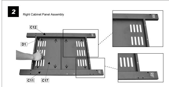
Attach the Right Legs (C11,C12) to the Side Panels (C17x2pcs) using ST4.0x10 Screws (D1x8pcs) as shown.
