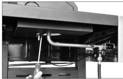
Feed the venturi tube of the Side Burner (C6) through the hole in bottom of the side burner shelf, and fix side it onto side burner shelf using a M4x10 Bolt (D2) as shown. Make sure that the end of venturi tube is set over the gas outlet of side burner valve.
