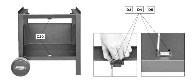
Attach the Magnets (C20) onto the bottom panel and upper support using M4x15 Bolts (D3x4pcs), Washer (D4x4pcs) and M4 Nuts (D5x4pcs) as shown.
