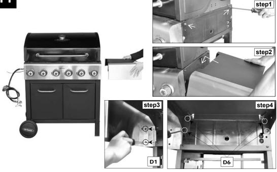
Attach the side shelf assembly to the barbecue body using ST4.0x10 Screws (D1x2pcs) and M6x15 Bolts (D6x4pcs) as shown.
