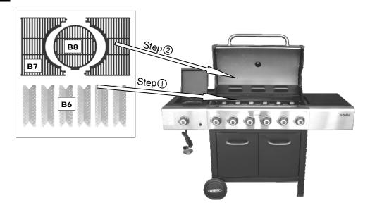
Carefully lay Flame Tamers (B6) into the barbecue body ensuring it lies level within the body. Lay the Cooking Grills (B7) and Round Grill (B8) into place.
