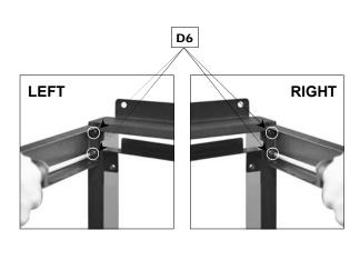
Attach the Upper Support (C14) between the front legs using M6x15 Bolts (D6x4pcs).
