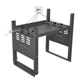
Complete fixing the left cabinet panel and right cabinet panel onto bottom panel using the ST4.0x10 Screw (D1x6pcs) as shown.
