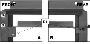
Attach the Drip Tray Left Bracket (B11) to the left legs using ST4.0x10 Screws (D1x2pcs) as shown. Repeat above process for Drip Tray Right Bracket (B12).
