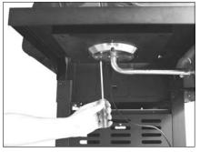
Feed the venturi tube of the Side Burner (C6) through the hole in bottom of the side burner shelf, and fix side it onto side burner shelf using a M4x10 Bolt (D2) as shown. Make sure that the end of venturi tube is set over the gas outlet of side burner valve.
