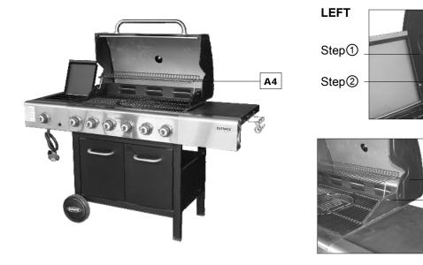
Attach the Warming Rack (A4) to the Hood (A1) and Barbecue Body (B1) as shown. Make sure that the swing legs fix to the body of the barbecue and the shorter fixed legs go through the holes in the hood.
