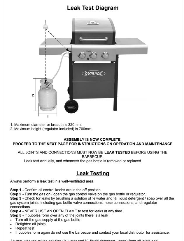
Always wipe the mixed solution ( $\frac{1}{2}$  water and  $\frac{1}{2}$  liquid detergent / soap) from all joints and connections after leak testing.
