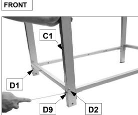
Assembly the Legs (C1, C2, C3, C4) and Leg Supports (C5, C6, C7) together using the M6x15 Bolts (D1x8pcs), M6x65 Bolts (D9x4pcs) and M6x40 Bolts (D2x4pcs) as shown.
