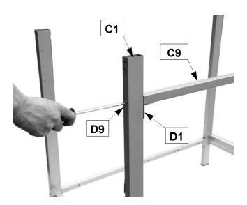
Attach the Trolley Support (C9) to the left front leg and right front leg using M6x15 Bolts (D1x2pcs) and M6x65 Bolts (D9x2pcs) as shown.
