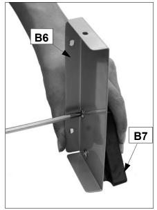
Attach the Rear Support Bracket (B4) to the Hood Rear Support (B5) using M6x8 Bolts (D4x2pcs). Attach the Front Support Bracket (B6) to the Hood Front Support (B7) using M6x8 Bolts (D4x2pcs) as shown.
