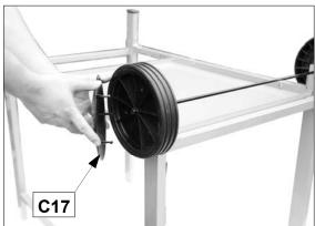
Unscrew the Locknuts (D10) from both ends of the Axle (C15). Slide the axle through the corresponding holes in the left legs. Slide the Wheels (C16) over each end of the axle. Secure the wheels into place with the locknuts. Place the Hubcaps (C17) onto the outsides of the wheels.
