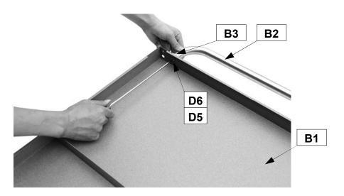
Attach Trolley Handle (B2) and Trolley Handle Sheaths (B3) to the Working Surface Assembly (B1) using M6x20 Bolts (D6x2pcs) and Ø8.5 Washer (D5x2pcs) as shown.
