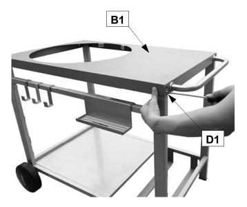
Attach the Working Surface Assembly (B1) to the trolley assembly using M6x15 Bolts (D1x8pcs) as shown.
