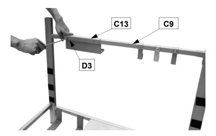
Attach the Knife Holder (C13) to the Trolley Support (C9) using ST4x10 Screws (D3x2pcs) as shown.
