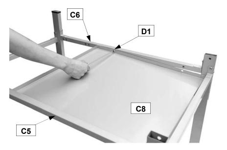
Attach the Bottom Shelf (C8) to the Leg Front Support (C5) and Leg Rear Support (C6) using M6x15 Bolts (D1x4pcs) as shown.
