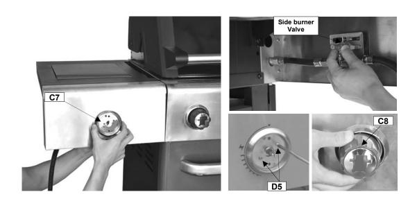
Attach the side burner valve and Knob Bezel (C7) onto side burner shelf using M4x10 Bolts (D5x2pcs) as shown. Press the Side Burner Knob (C8) onto side burner valve stem.
