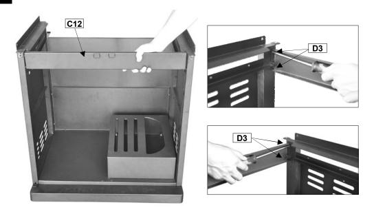
Attach the Upper Support (C12) to the left/right cabinet panel using M6x15 Bolts (D3x4pcs).
