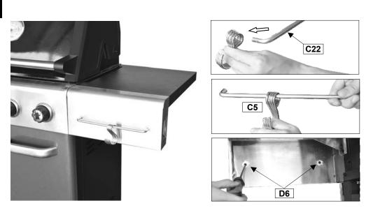
Insert the Hook Rail (C22) through the Tool Hooks (C5) as shown, then fix the assembly onto side shelf panel using M5x10 Bolts (D6x2pcs).
