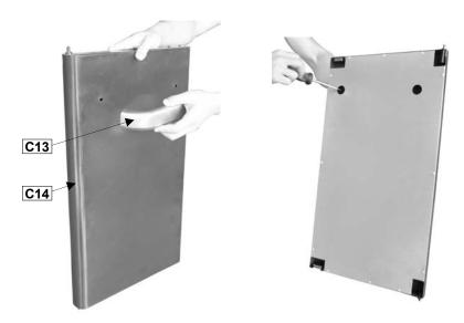
Remove the retaining bolts from one Door Handle (C13), then attach the door handle onto the Left Door (C14) using the retaining bolts as shown. Repeat above process for the Right Door (C15).
