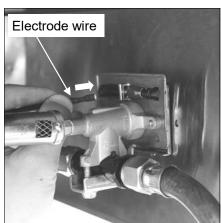
Connect the electrode wire to the ignitor.
