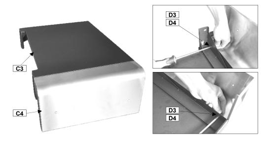
Attach Side Shelf Panel (C4) onto Side Shelf (C3) using M6x15 Bolts (D3x2pcs) and M6 Nut (D4x2pcs) as shown.
