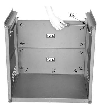
Attach the Rear Panels (C16) onto the cabinet assembly using ST4.0x10 Screws (D2x11pcs) as shown.
