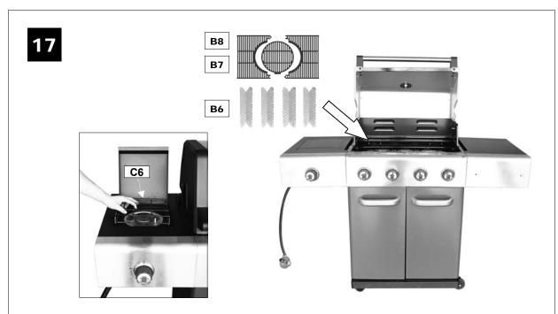
Lay the Flame Tamers (B6) carefully into the body ensuring it lies level within the body. Lay the Cooking Grills (B8) and Round Grill (B7) into place. Place the Side Burner Grid (C6) onto the side burner shelf.
