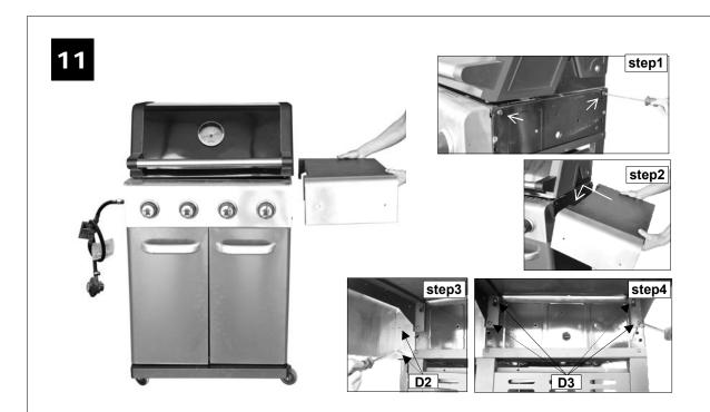
Attach the side shelf assembly onto the barbecue body using ST4.0x10 Screw (D2x2pcs) and M6x15 Bolts (D3x4pcs) as shown.
