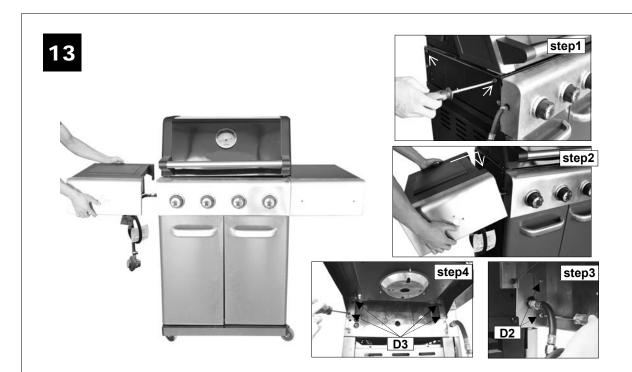
Attach the side burner shelf assembly onto the barbecue body using ST4.0x10 Screw (D2x2pcs) and M6x15 Bolts (D3x4pcs) as shown.
