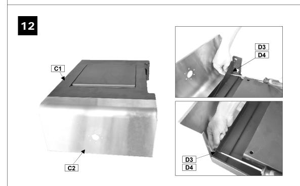
Attach Side Burner Shelf Panel (C2) onto Side Burner Shelf (C1) using M6x15 Bolts (D3x2pcs) and M6 Nut (D4x2pcs) as shown.
