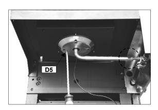
Feed the venturi tube of the Side Burner (C9) through the hole in bottom of the side burner shelf, and fix it by using a M4x10 Bolt (D5) as shown. Make sure that the end of venturi tube is set over the gas outlet of side burner valve.
