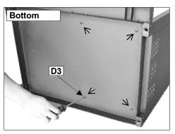
Attach the Storage Unit (C19) onto the bottom panel using M6x15 Bolts (D3x4pcs) as shown.
