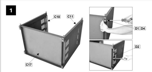
Attach the Left Cabinet Panel (C10) and Right Cabinet Panel (C11) to the Bottom Panel (C17) using M6x35 Bolts (D1x8pcs), M6 Nuts (D4x8pcs) and ST4.0x10 Screw (D2x6pcs) as shown.
