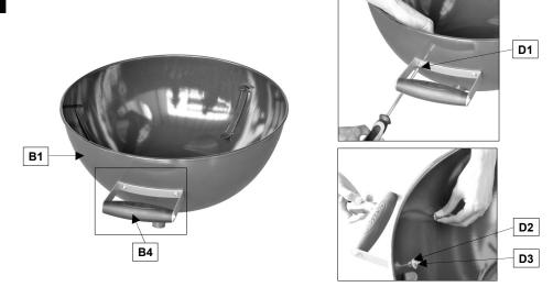
Attach the Body Handle (B4) onto the Barbecue Body (B1) using the M6x15 bolts (D1x2pcs), M6 washers (D2X2pcs) and M6 Nuts(D3x2pcs) as shown.
