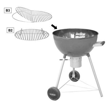
Place the Charcoal Grill (B2) onto the lower brackets in the barbecue body. Ensure the charcoal grill lies level within the body.
