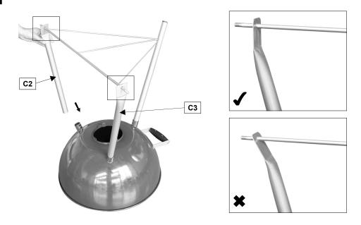
Slide the Right Rear Leg (C3) onto straight bar of the leg support rack. then insert the other end of right rear leg into the leg support of the barbecue body, as shown. Repeat above process for the Left Rear Leg(C2).
