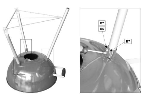
Secure by the M5x15 Bolts (D5x6pcs) through the M5 Washers(D7x6pcs), Body Gaskets (B7) and leg support of the barbecue body into the legs.
