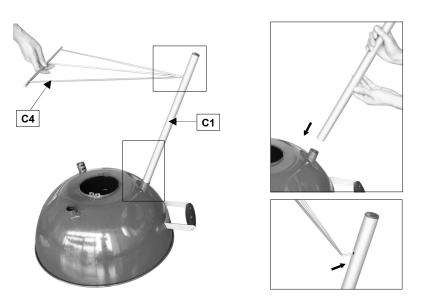
Insert the Front Leg (C1) into the leg support of the barbecue body. then insert the angled end of Leg Support Rack (C4) into the end hole near the end of the front leg.
